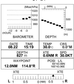
Figure 2-22 Navigation data display during stand-by
